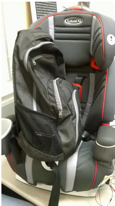
Fig. 20. Force Sensor detecting backpack as a child
